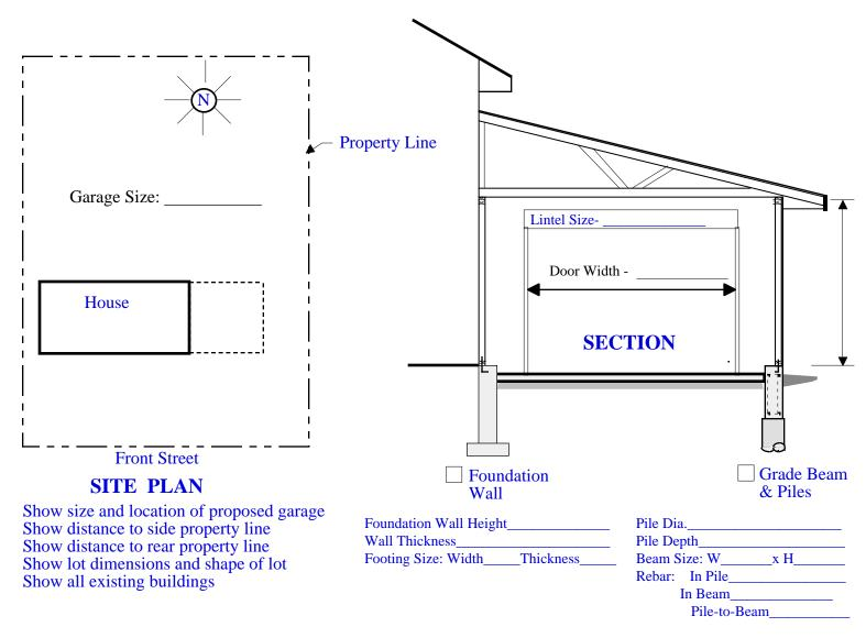
Note: The foundation must extend to the same depth or greater than the house foundation.
